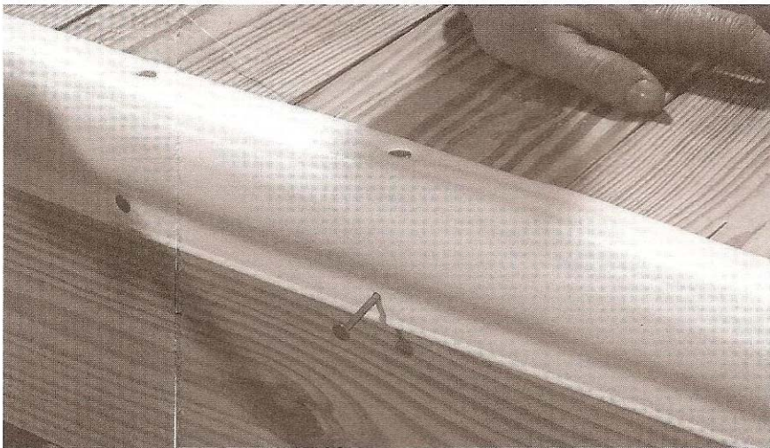
31. Attach rubrail using the same stainless nails. We recommend a nail every 6" top and bottom.
